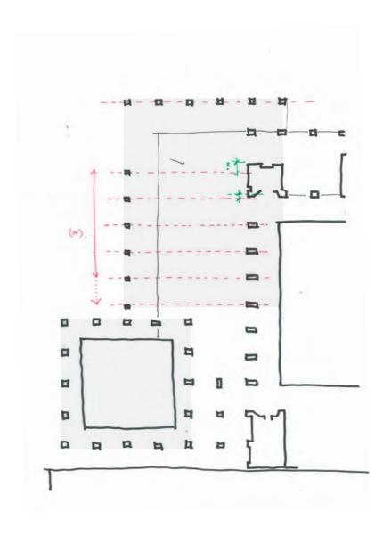
3 Uniform columns at facade Set-out in line with existing columns
