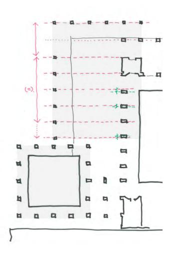
4 Uniform columns at facade Set-out eccentric to existing columns
