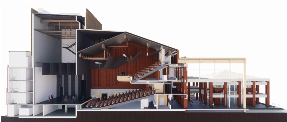
Figure 2.2: Sectional perspective of Sutherland Entertainment Centre
