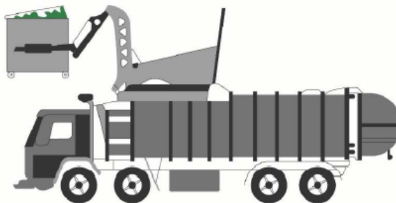
Front-lift-loading waste collection vehicle
