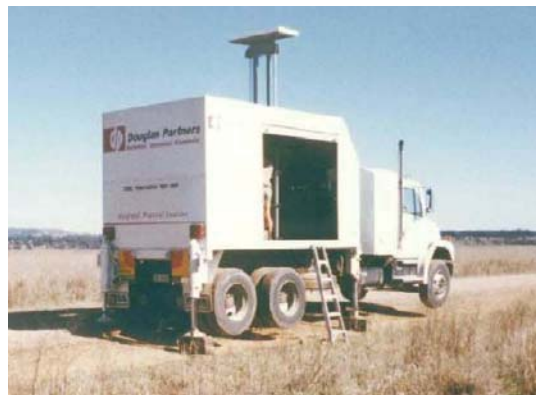
Figure 2: Purpose built CPT rig
