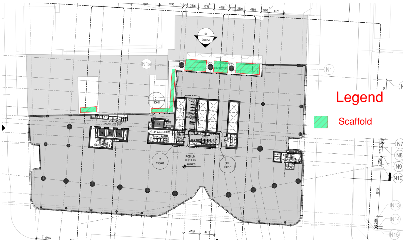
Figure 30 – Plan View - Scaffolding & Screens Alongside Ashington Place & Masonic Club (levels 5-9)
