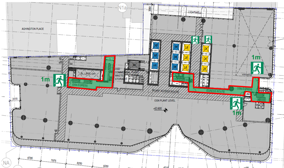
Figure 22 Exits from OSD plant level 9
