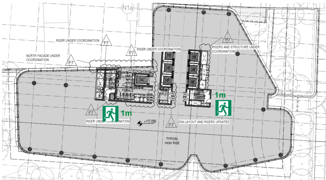
Figure 24 Exits from typical high-rise level
