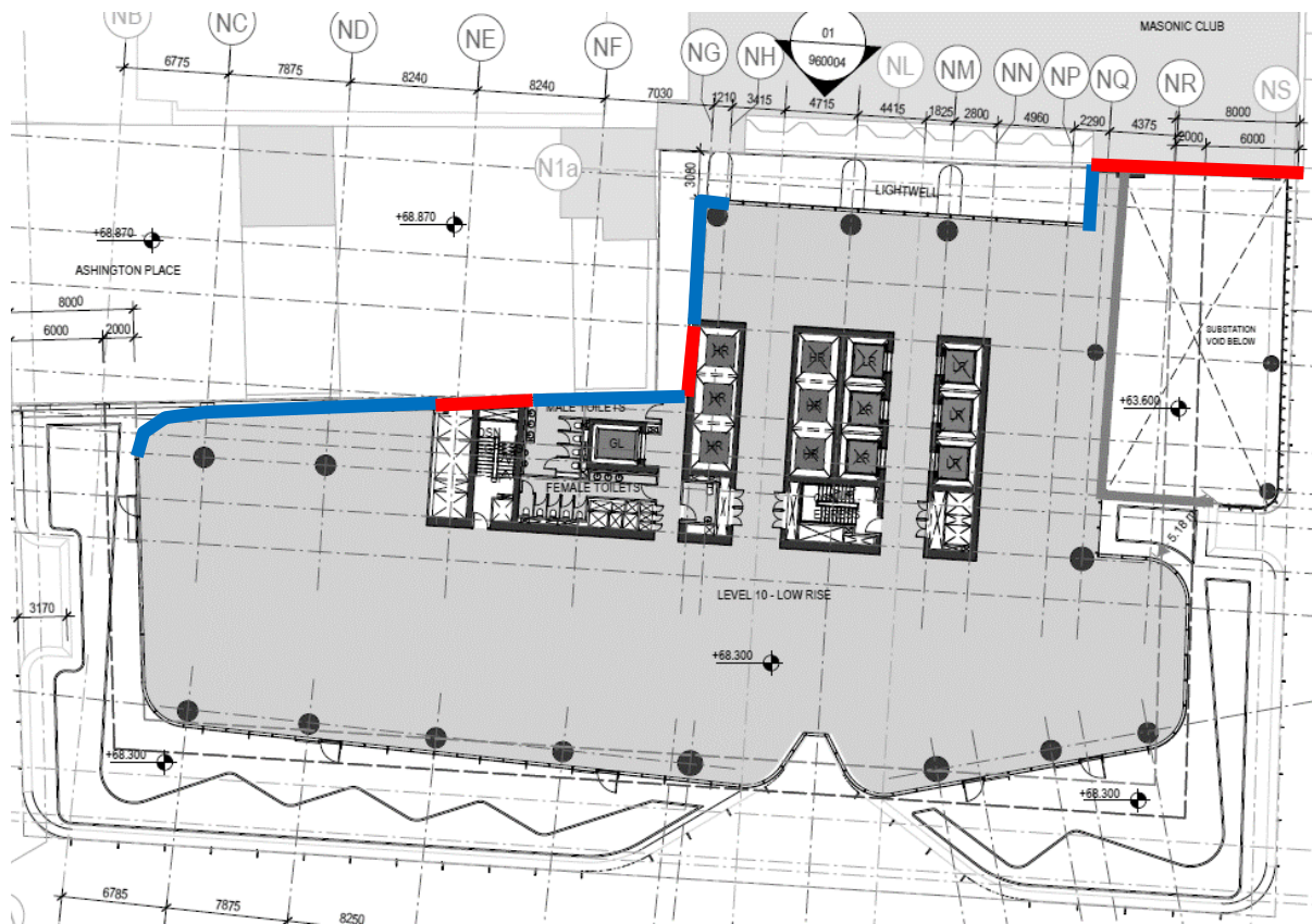
Figure 12 Indicative protection of external walls of OSD low-rise level 10
