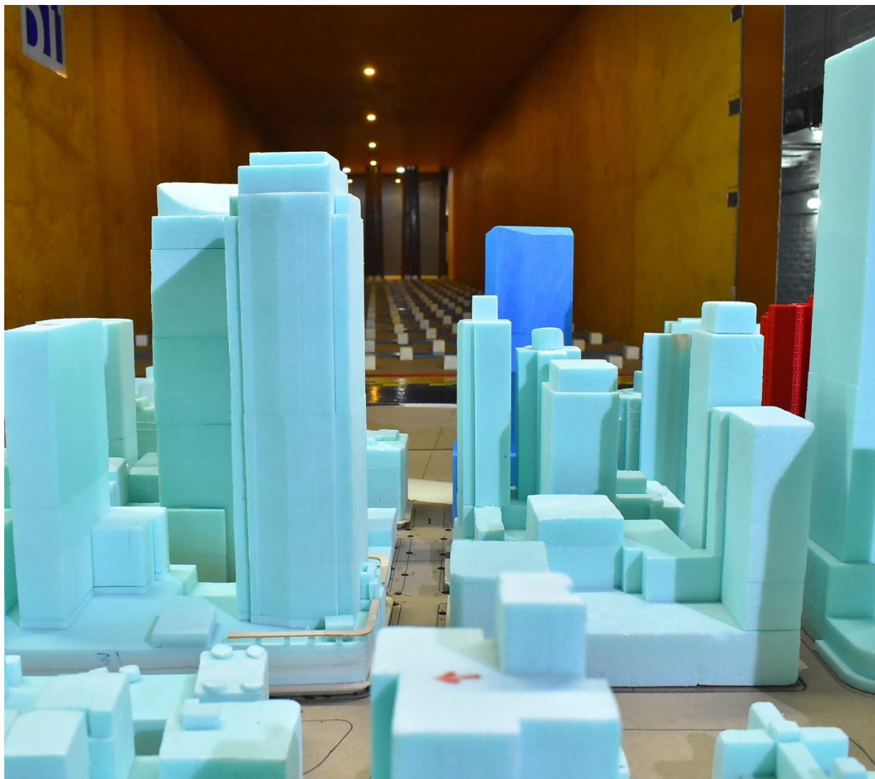
Image 2B: Wind Tunnel Study Model – Existing Site with 210 Elizabeth Street Stage 1 DA Massing Envelope Configuration
