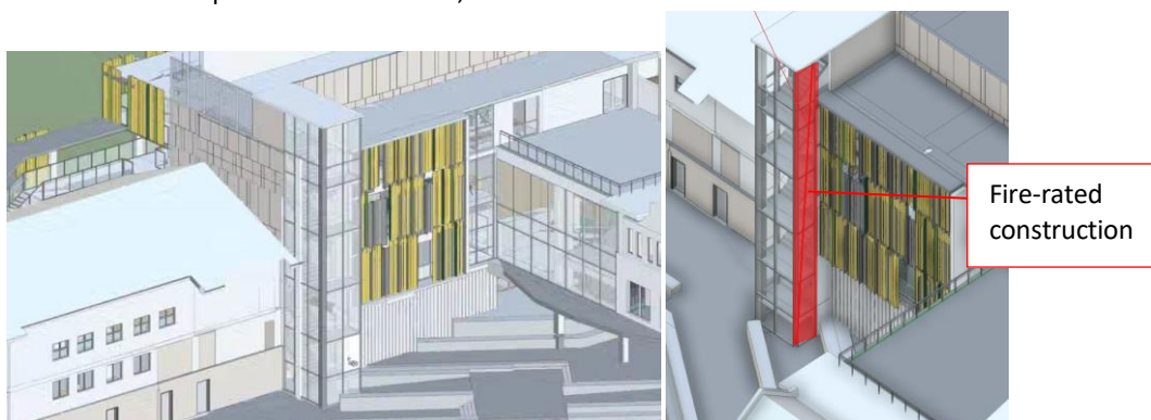
Figure 0.5: Stairway to generally be located within a fire-isolated shaft where glazed external construction shall comply with Clause C3.8
