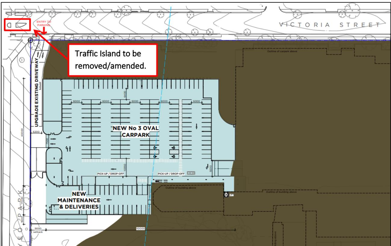
Figure 4-4 New Primary Maintenance & Delivery Area
