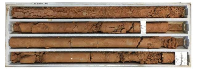
Figure 9: UG-BH-02 core photo showing Lake Sediments (13.0 m - 18.9 m)
