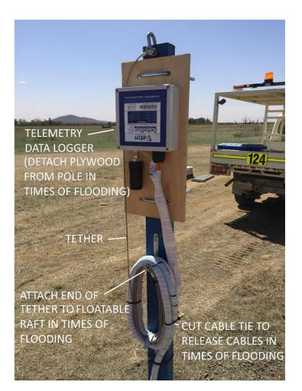
Figure 7: Telemetry installation
