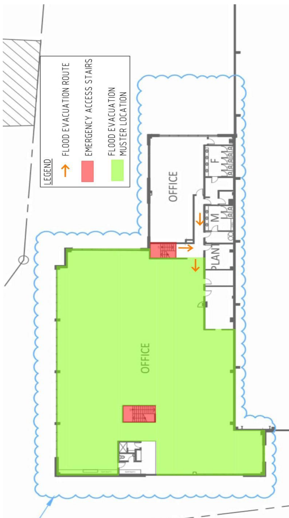
Figure 3 – First Floor Evacuation Route & Safe Refuge Area
