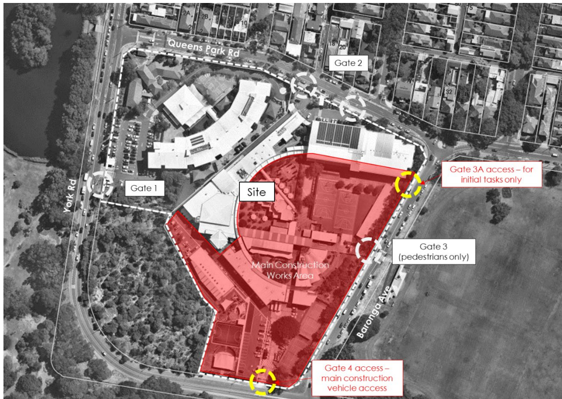
Figure 3.2: Proposed Construction Site Access Gates
