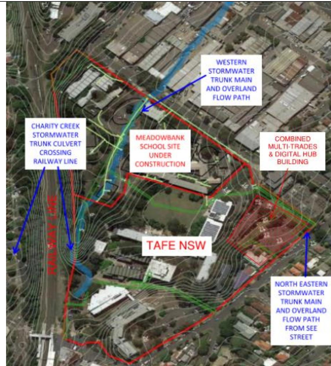
Figure 3.1.2: Meadowbank TAFE Stormwater Network
