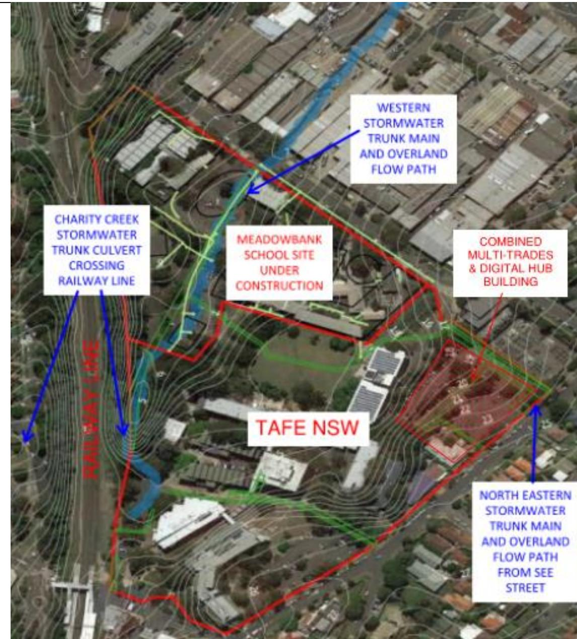
Figure 3.1.2: Meadowbank TAFE Stormwater Network
