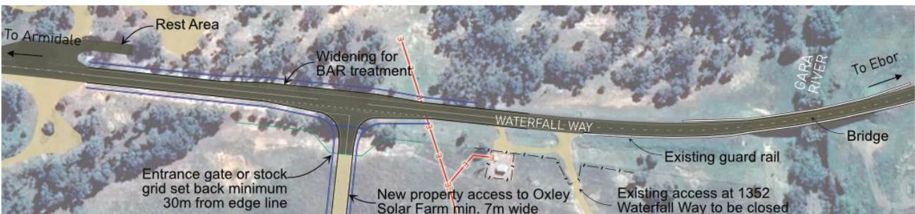
Figure 4-11 Concept Diagram of new property access arrangement to Waterfall Way (Grafton Road) (New England Surveying & Engineering, 2020).
