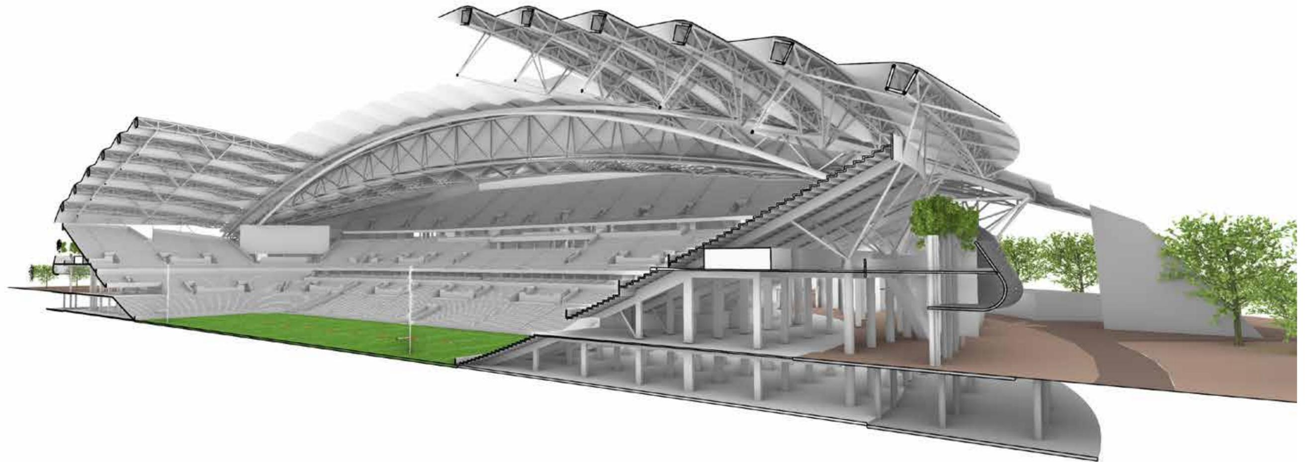
Figure 27: Longitudinal Section Looking at the West Stand
