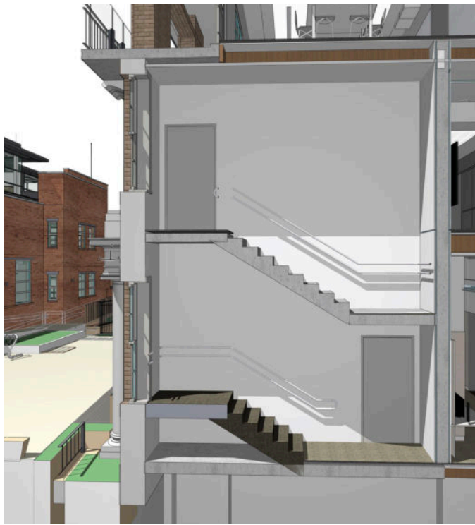
/ S4.55 / West 3D Sectional View - New Stair
