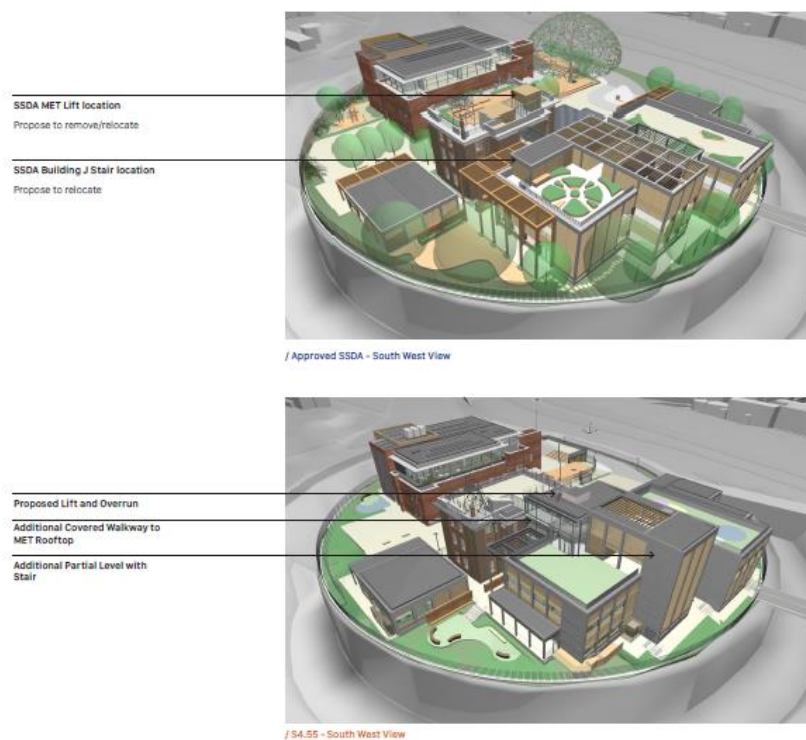
Figure 4 Removal and relocation of the Met Building lift
