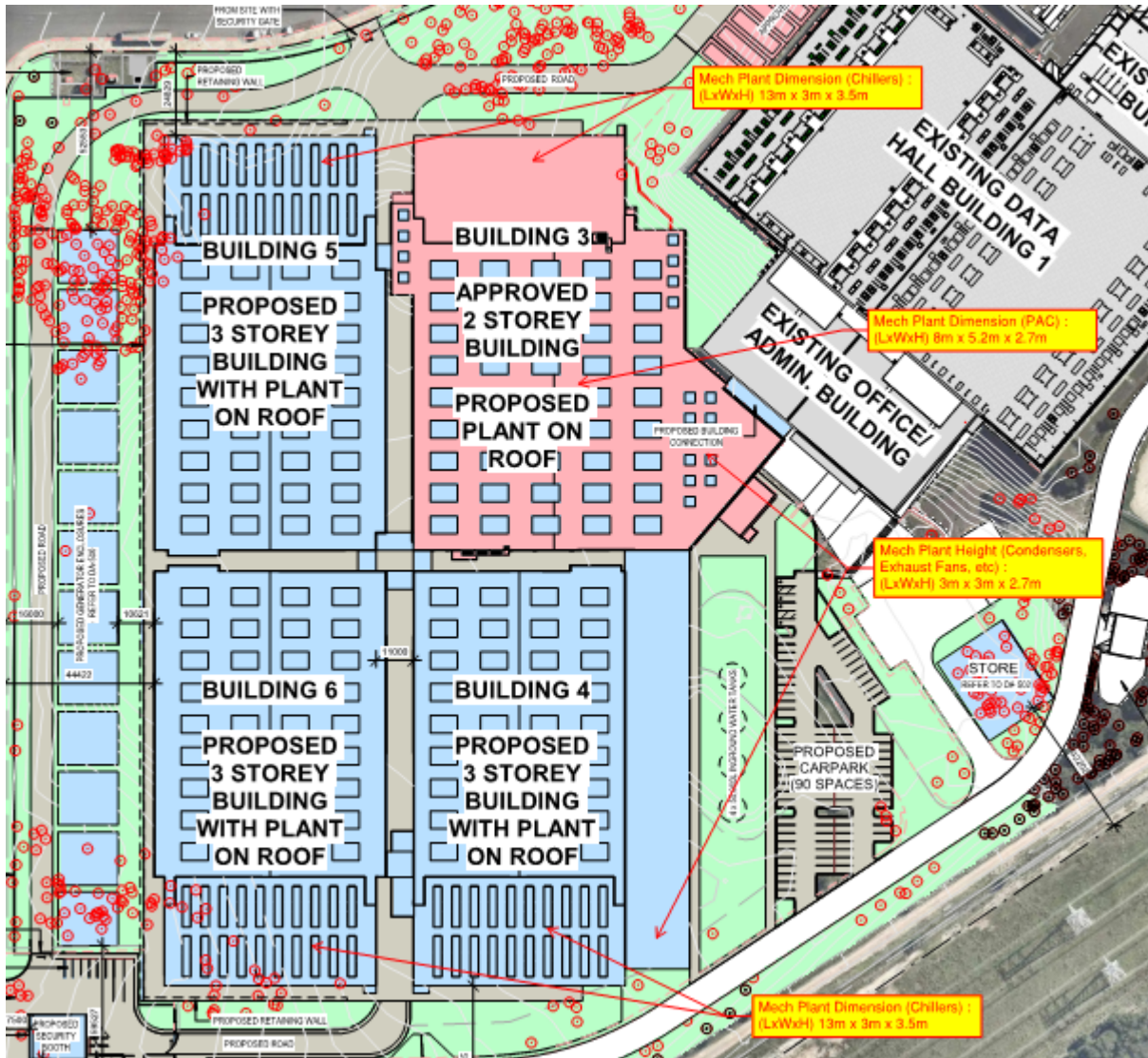
Figure 6 : Proposed Mechanical Plant on roof of Buildings 3,4,5 & 6
