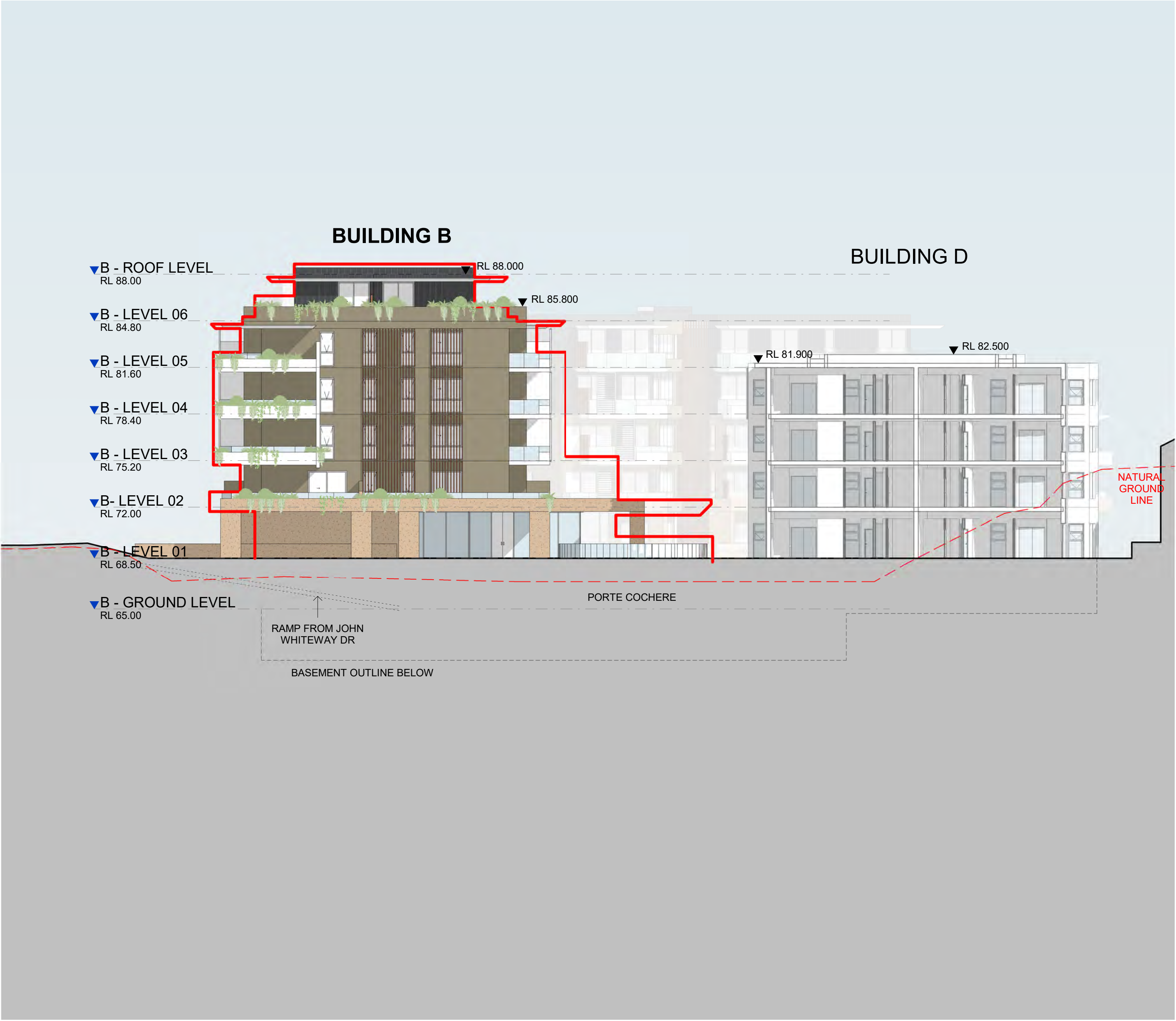
1 BUILDING B - NORTH ELEVATION 1 : 200
