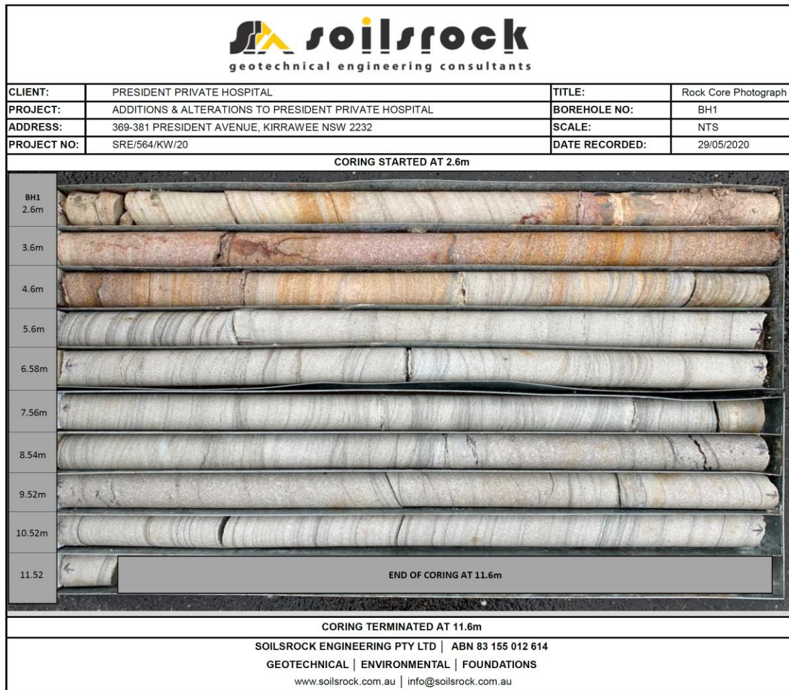
Figure 5.17 Geotechnical Bore Log BH1 - Rock Core Photograph. Soilsrock Engineering Pty Ltd, 2020.
