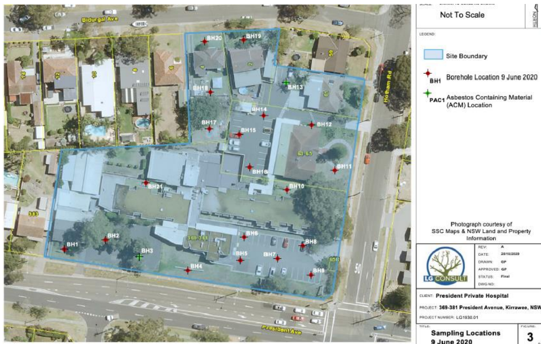
Diagram 12: Location of Boreholes and Asbestos Containing Material.
