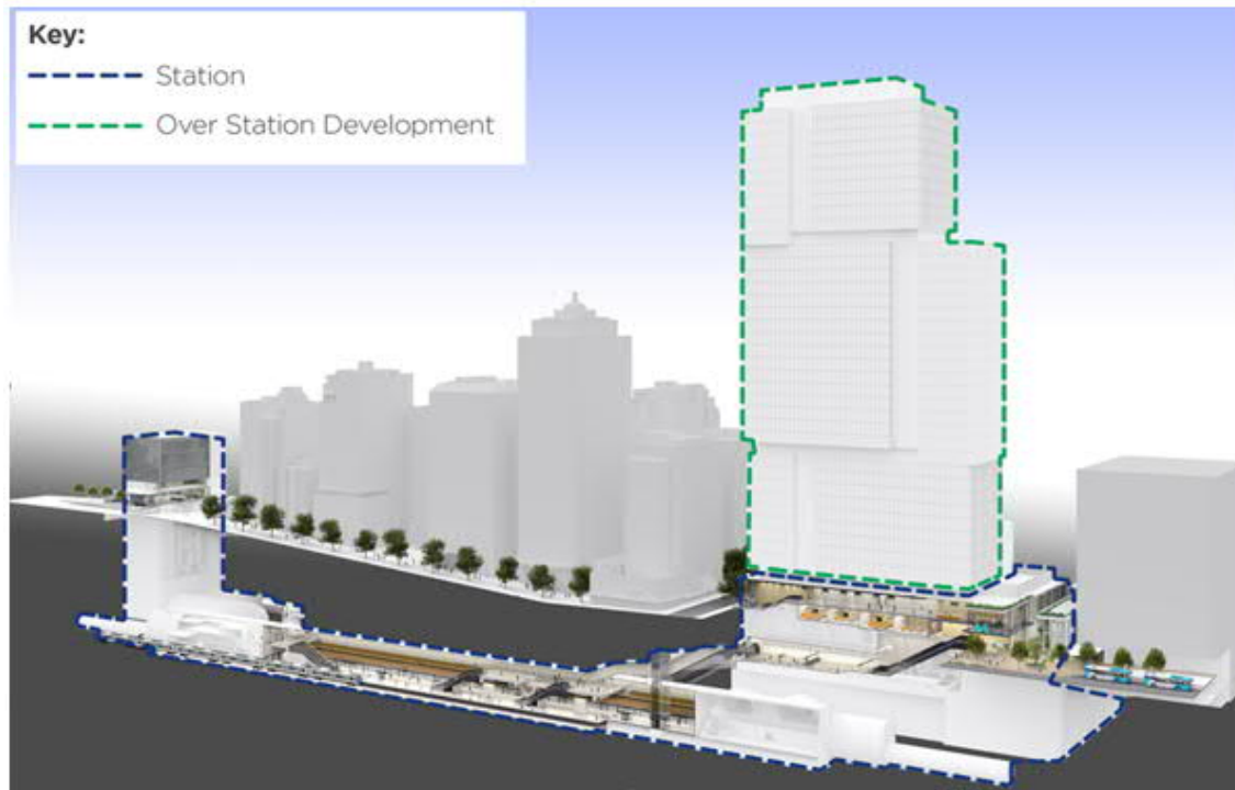
Figure 3-1 Schematic 3D View of the ISD Showing OSD & Station Components
