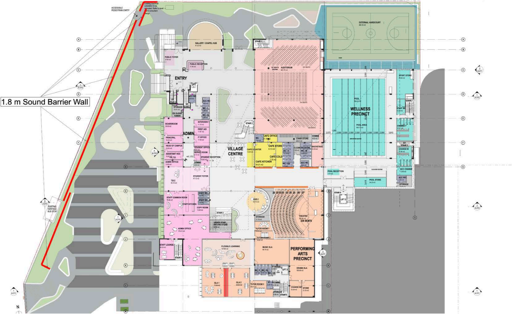
Recommended Sound Barrier Wall Location
