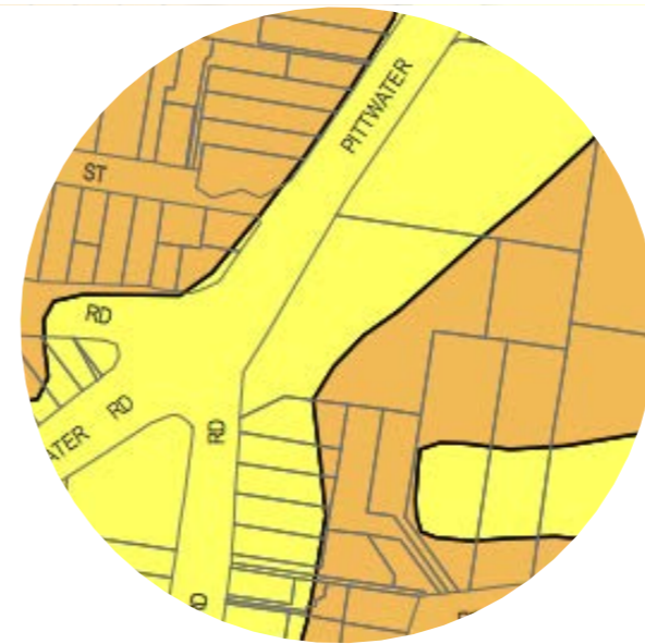
Landslip Risk Map Categories A (yellow) + B (orange). A = slope < 5° B = Flanking Slopes 5° - 25°
