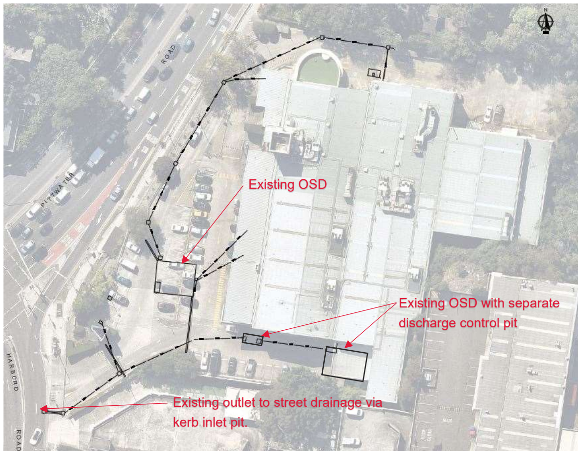
Figure 2 - Pittwater Road Existing Stormwater Infrastructure
