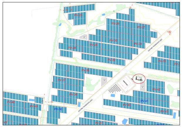
Figure 3-21 The proposed location of temporary construction facilities, east of the proposed substation.
