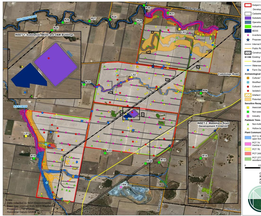
Figure 3-8 Proposal infrastructure layout and site environmental constraints
