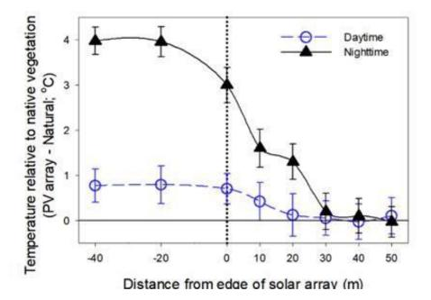
Figure 7-2 Measures of air temperature within and outside of the PV array (source:- Barron-Gafford 2016)
