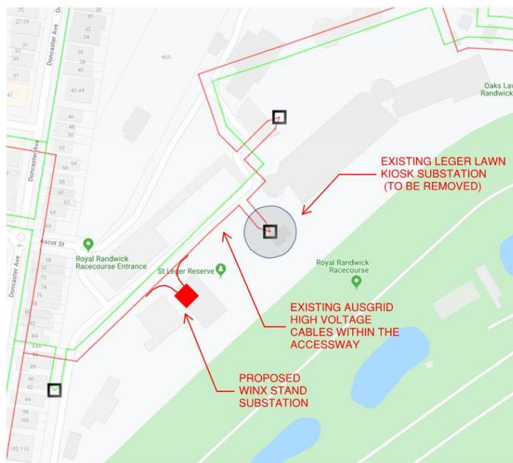
Figure 2: Existing Ausgrid high voltage cables and substation alterations (approximate locations)
