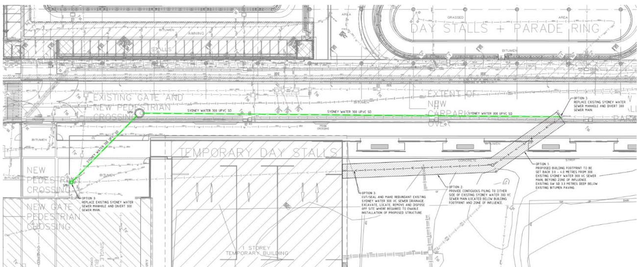
Figure 2: Proposed Sydney Water sewer main diversion works.
