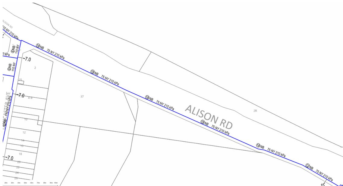
Figure 3: Existing Jemena Gas reticulation main.
