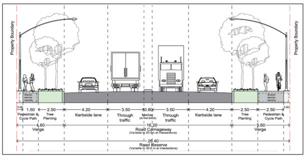
Figure 11: Draft DCP Typical Distributor/Collector Road Source: Mamre Road Precinct Draft DCP 2020
