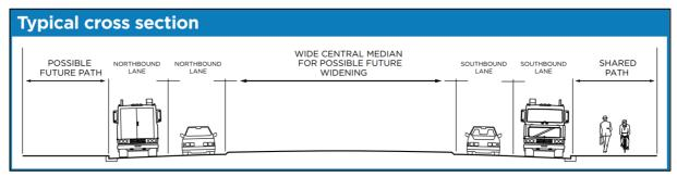
Figure 6: Mamre Road Upgrade Typical Cross Section
