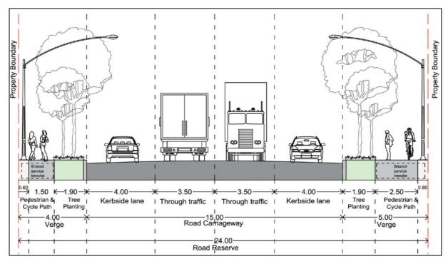
The proposed Access Roads would eventually form a High Order Road under the Draft DCP. The preferred cross-sections within the Draft DCP are shown by the below figures.
