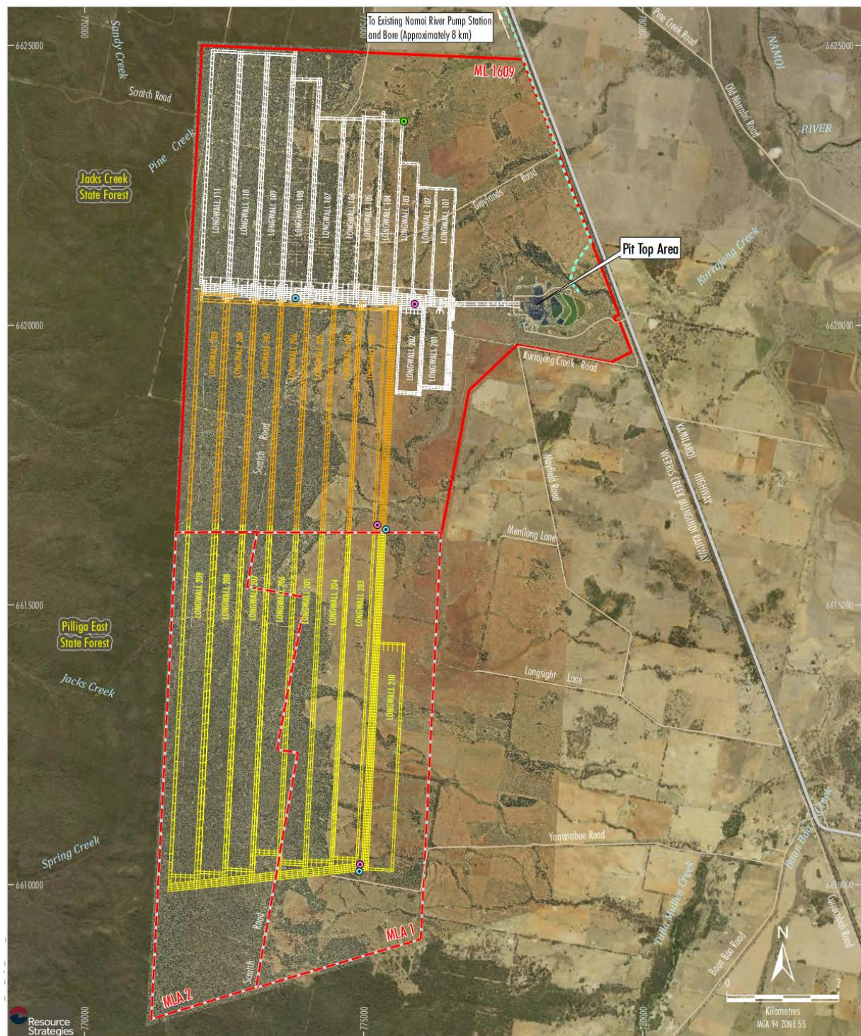
Figure 2 - Project Indicative Underground Mining Layout (Source: Applicant's Amendment Report)
