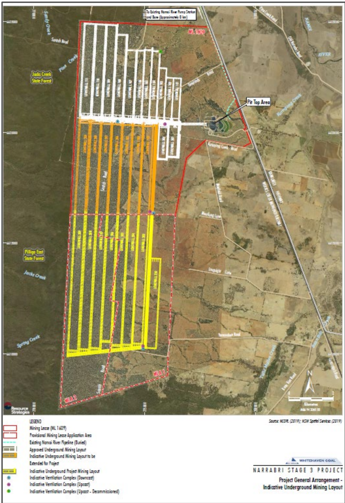
Figure 2 | Project Longwall Layout (Source: EIS)
