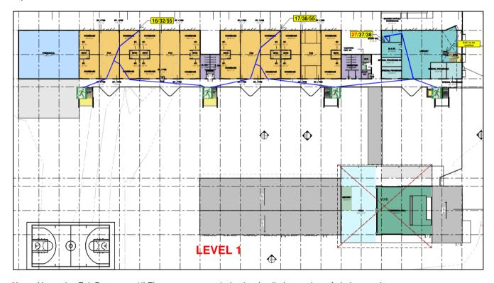
Note: Alternative Exit Routes on 1st Floor area are needed to be detailed, as points of choice need to egress through other home base and sliding doors, so latching and exit sign detailing to be provided Note 2: Circulation stair in Library is not an exit, and for BCA Compliance cannot be used as an exit...
