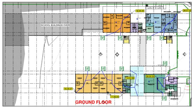
Note: Alternative Exit Routes on Ground Floor area are needed to be detailed, as points of choice need greater seperation.
