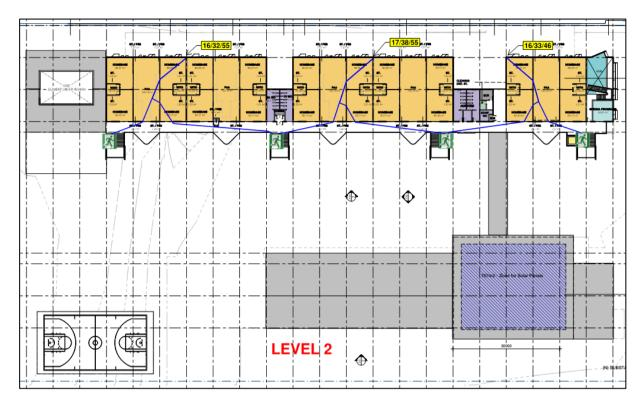
Important Note: In order to achieve the 20m to a point of choice, egress splits internally with the Home bases / Buildings as indicated - this will need to be coordinated with Architect (door latching/provision), Electrical Consultant for Exit sign locations to indicate alternative egress paths and security to ensure doors in paths of travel are not secured and provided with 24/7 egress as no Fail Safe release is possible in this school.
