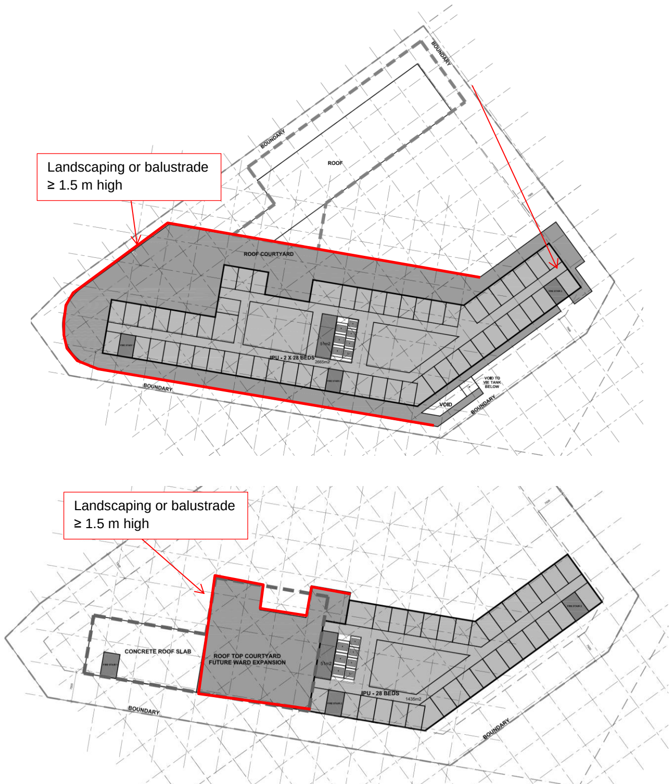
Figure 9: Recommended wind control treatments for Level 3 and Level 5
