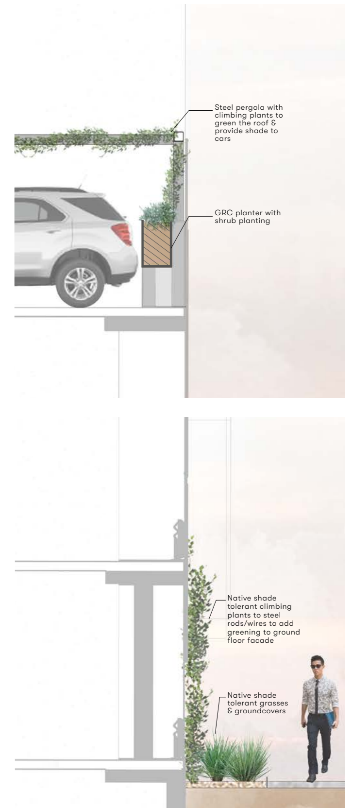
Figure 13 Ground & Rooftop Facade Section
