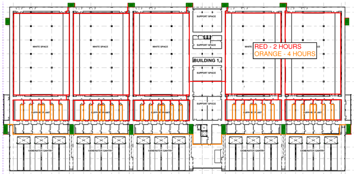
Figure 5-3: Fire compartmentation Plan on upper levels – Building 1
