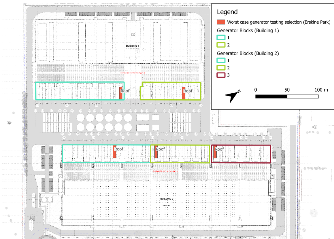
Figure 8-5: Generator testing configuration for the worst-case receiver specific in Erskine Park
