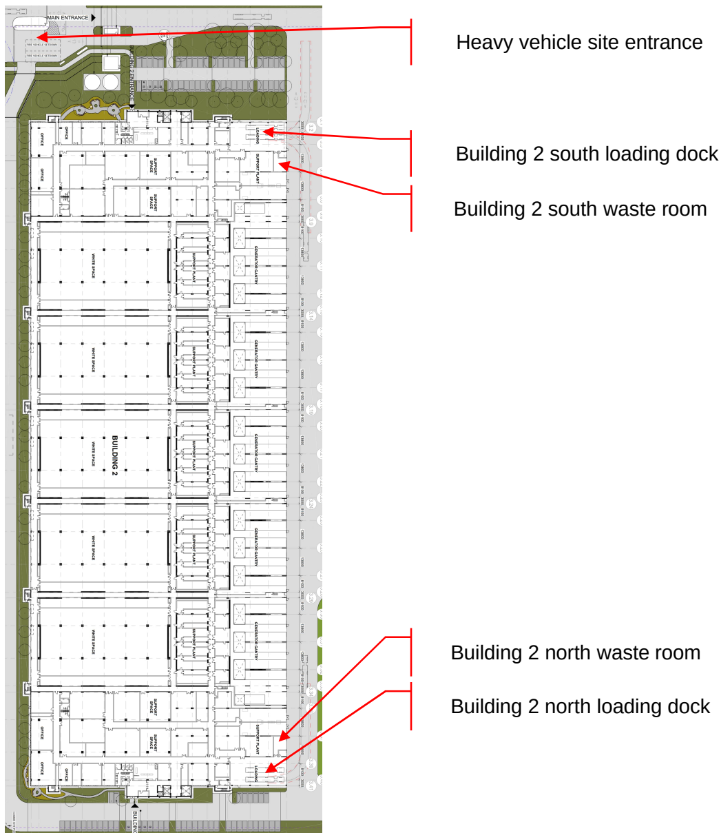
Figure 8 – Building 2 loading dock and waste room with heavy vehicle access
