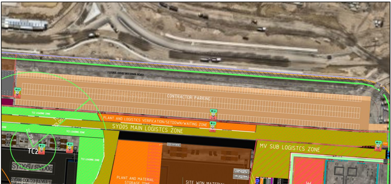
FIGURE 4: 504 CAR PARKING SPACES IN CONTRACTOR PARKING AREA
