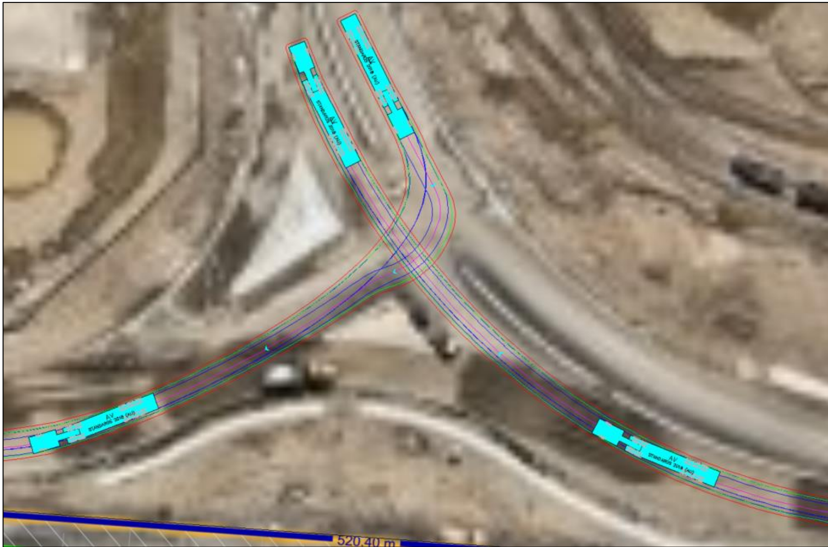
AV ENTRY AND EXIT FROM PUBLIC ACCESS ROAD ALONG NORTHERN SITE BOUNDARY
