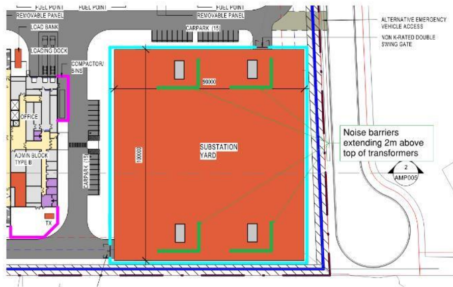
Figure 4: Indicative site transformer noise barrier locations
