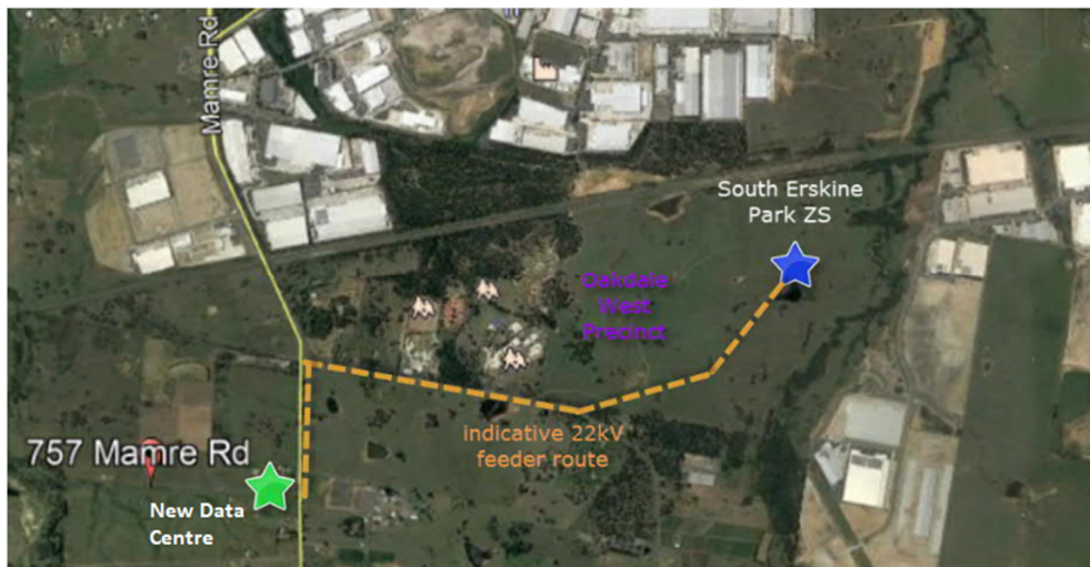
Figure 11 Interim 22kV supply from future South Erskine Park ZS (source Endeavour Energy 2020)
