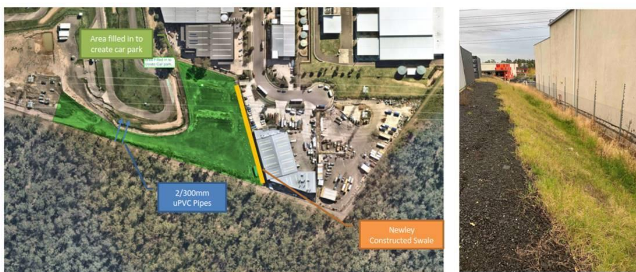
Figure 2 Aerial image of Event Carpark & Pit Area post-construction; area shaded green has been filled approximately up to 3.5m
