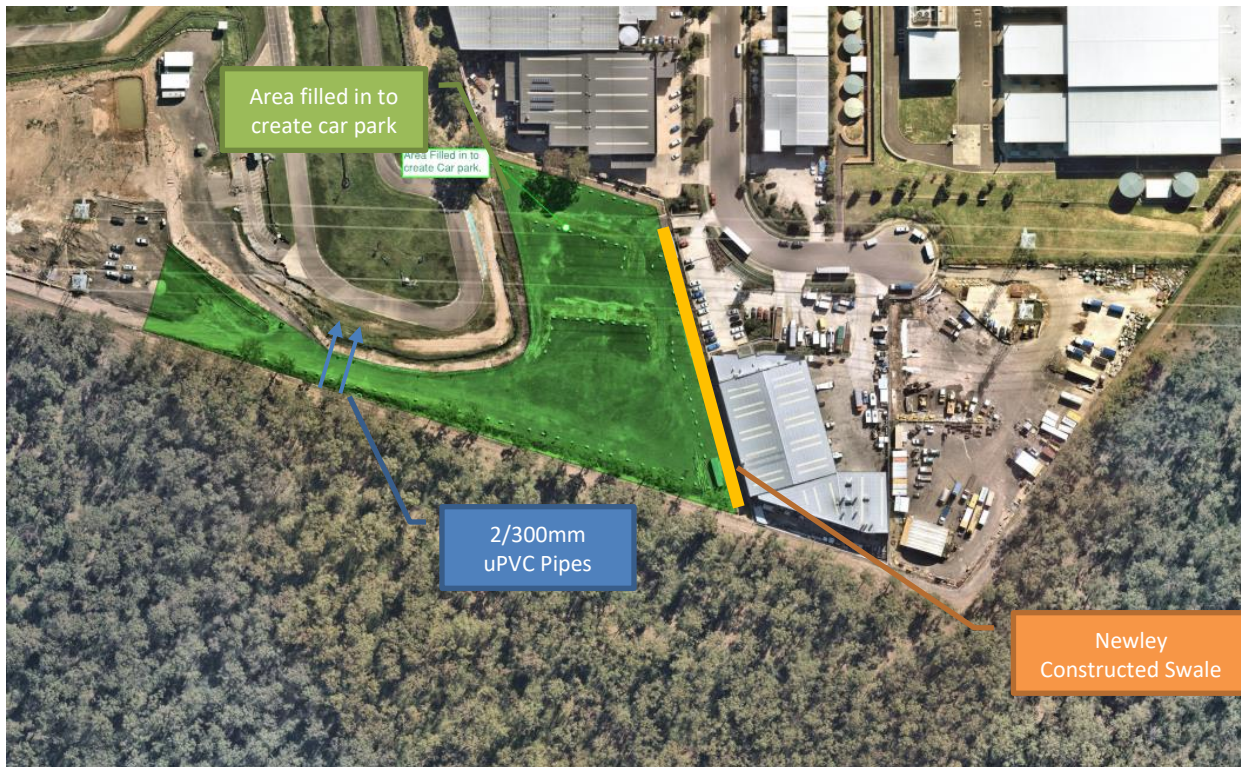
Figure 2 Aerial image of Event Carpark & Pit Area post-construction; area shaded green has been filled approximately up to 3.5m
