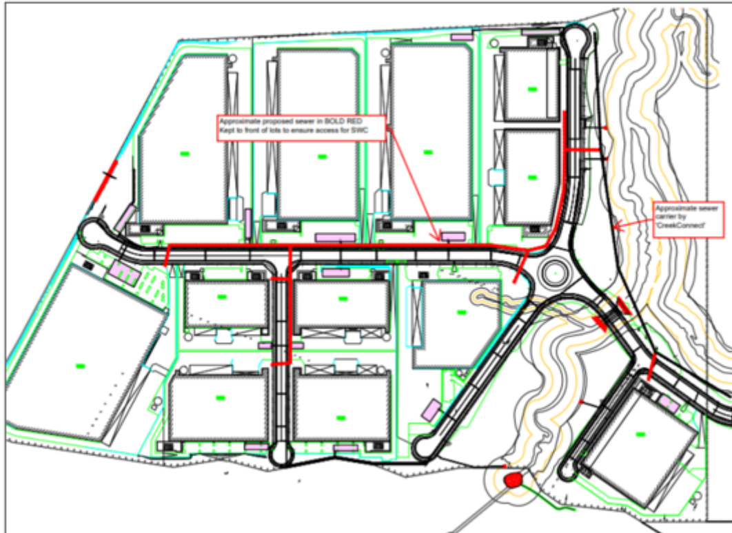
Figure 4 – Proposed sewer reticulation inside the development (developer)
