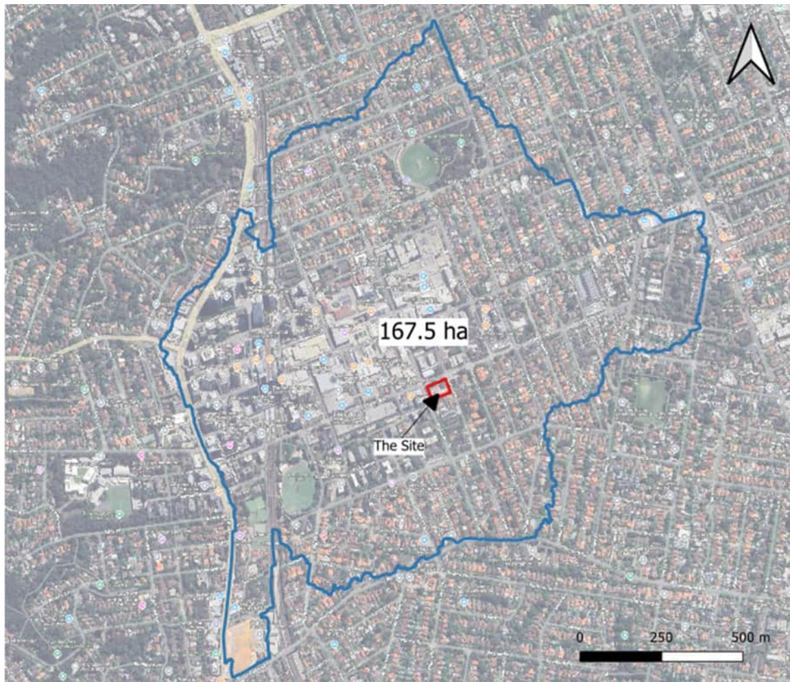
Figure 6: Catchment used to estimate Down Stream Boundary Condition of the TUFLOW model (Image source: Google Satellite Hybrid)
