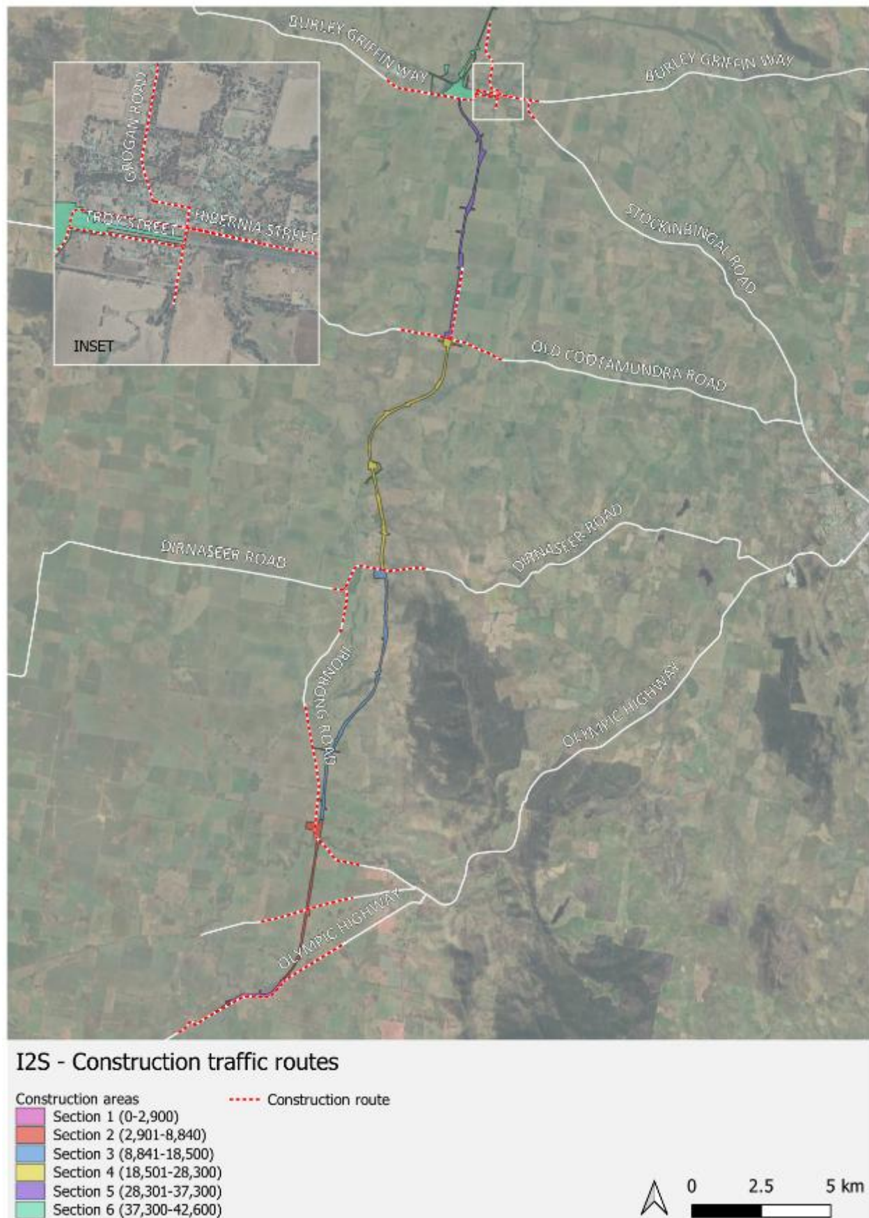
Figure 8-1 Construction traffic routes
