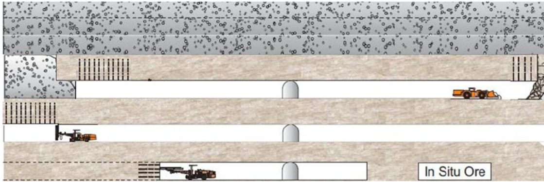
Figure 3-1 Underhand (top-down) longhole stoping with backfill mining method schematic
