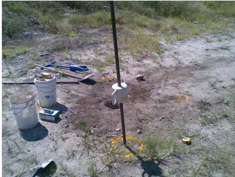
Plate 1: Temporary soil gas probe installation at BH_H4.
