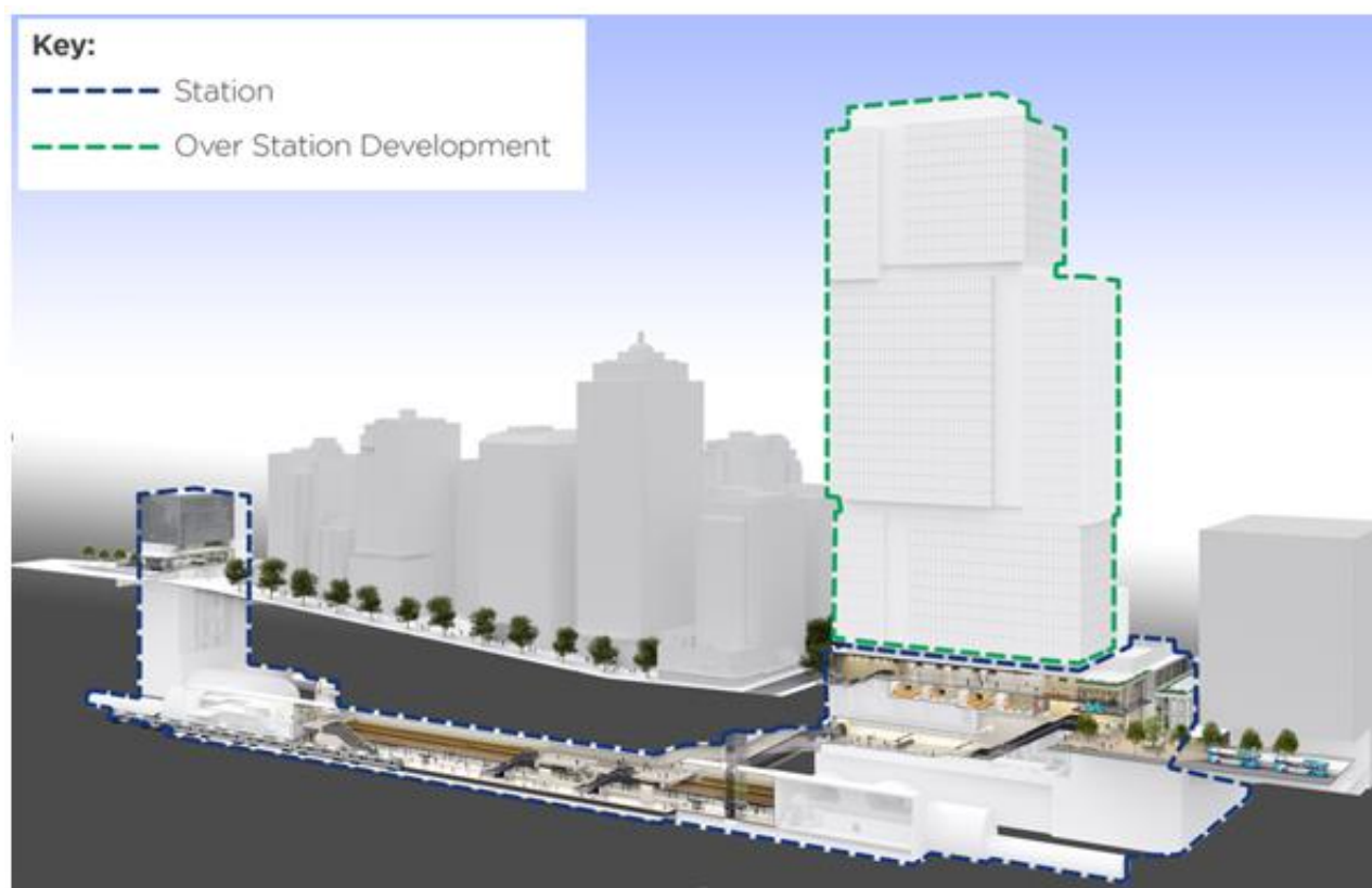
Figure - Schematic 3D View of the ISD Showing OSD and Station Components. Note: Northern (McLaren Street) station entrance shown on left, Southern (Berry Street) entrance shown on right.
