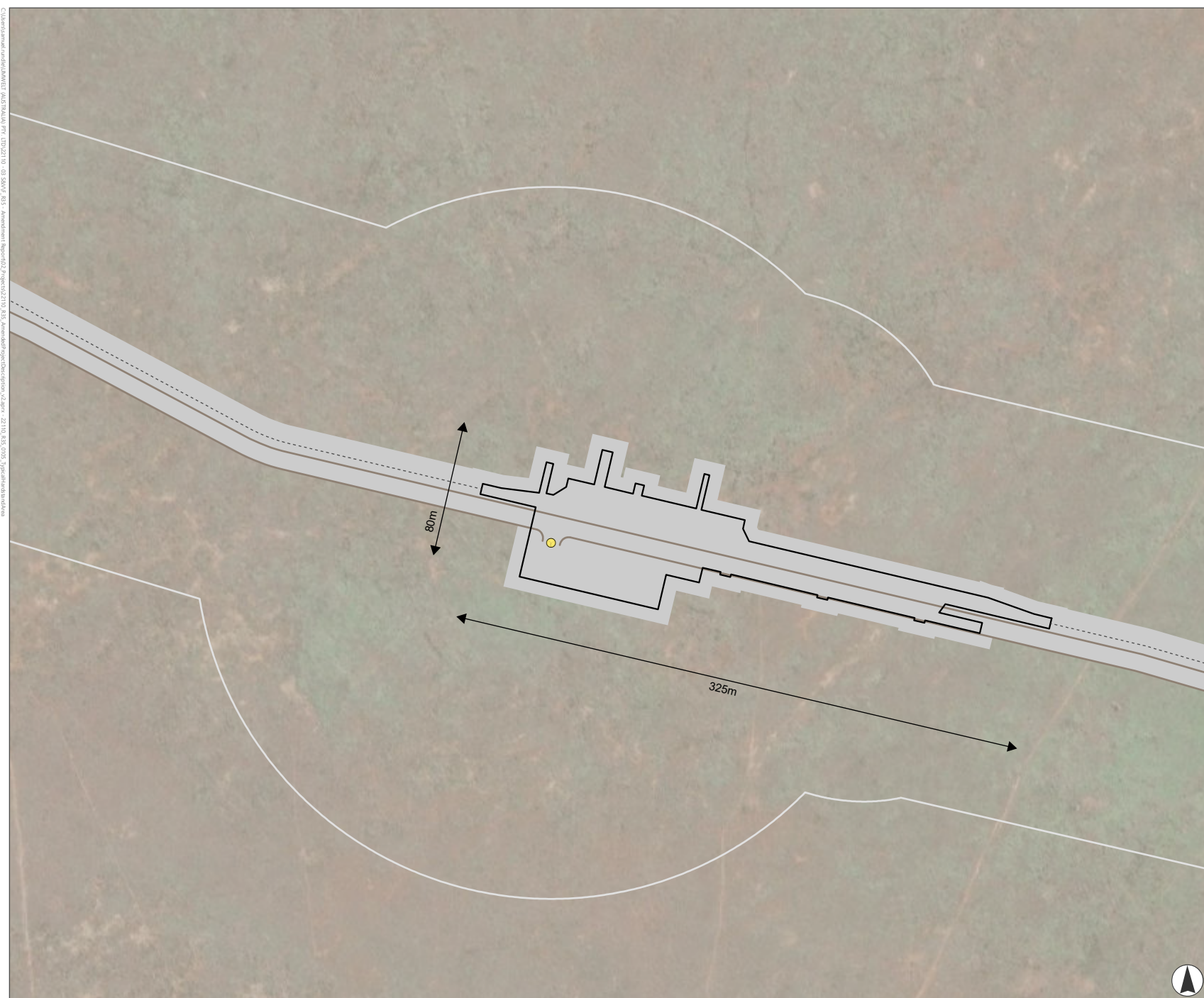
FIGURE 1.5 Typical Hardstand Area
