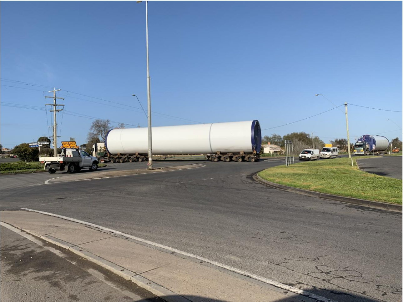
Photo 1.7 Delivery of Typical WTG Tower
