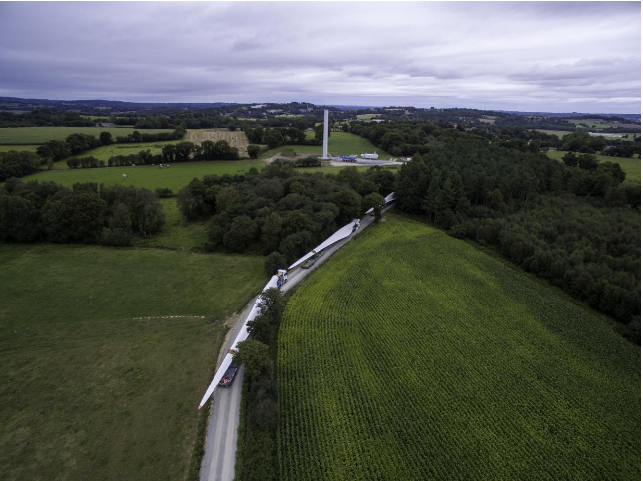
Photo 1.8 Typical Delivery of WTG Blades
