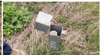
Groundwater Monitoring well LC2 near stream, offsite to the north of Bulga Mine. Well-cap missing.
