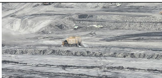
Water truck in operation within mine void
