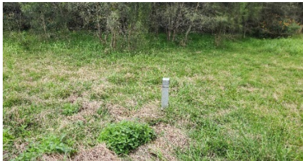
Groundwater Monitoring well LC2 near stream, offsite to the north of Bulga Mine. Well-cap missing.
